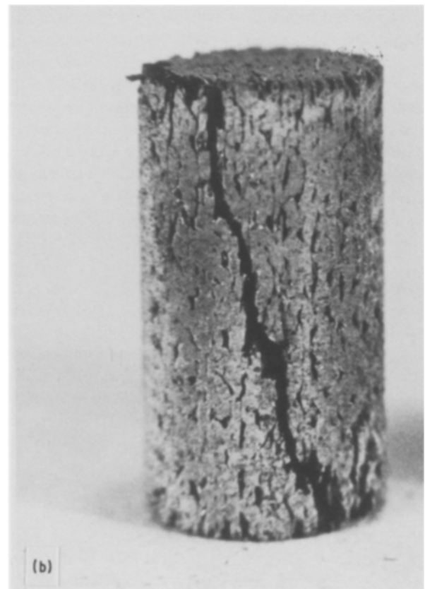
Figure 20 Failure modes of 2D-C-C/ceramic composites loaded in p -compression (a) low densification state, (b) full densification state.
