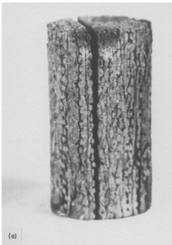
Figure 20 Failure modes of 2D-C-C/ceramic composites loaded in p -compression (a) low densification state, (b) full densification state.
